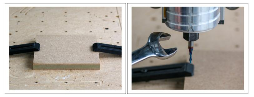
Clamp your selected material to the Spoilerboard of your WorkBee CNC Machine and hold in place using your chosen method this could be any of the following: Screws, Clamps with Tee Nut Waste Board or T-Track.
