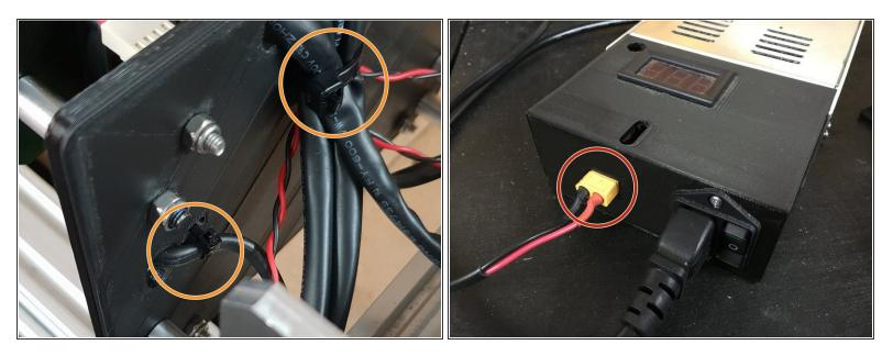
Using the already inserted cable ties fix the wires into place securely to prevent any unnecessary movement and to keep the machine looking neat!
