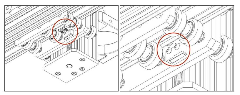
• Attach the Z-Axis limit switch to the threaded holes on the X-Plate-Front using 2 x M3- Socket-Head-10mm bolts, in the same orientation as the picture.
