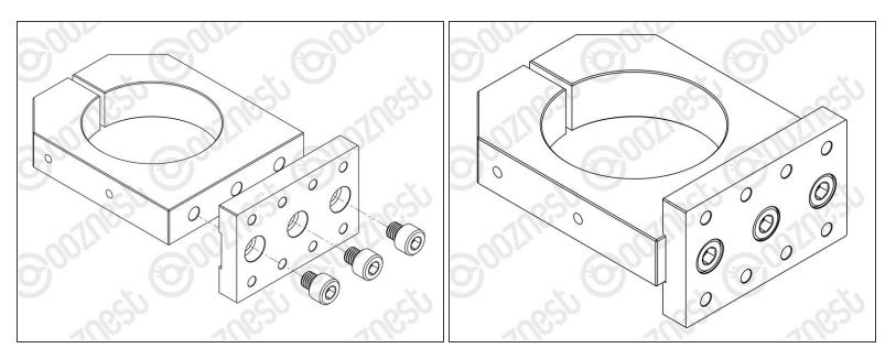
Attach the Z-Bracket to the Router-Clamp using 3 x M8-Cap-Head-Bolt-8mm. (Please note in your kit these may be M8-Cap-Head-Bolt-10mm)
