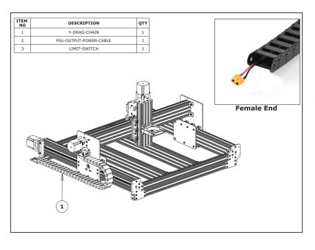
Lay the Y-Drag-Chain flat on a table. Feed the PSU-Output-Power-Cable through the whole length of the Y-Drag-Chain. Ensure that the end with the XT60-Connector, is located at the female end of the Y-Drag-Chain. (as shown in the 'Female End' image).
