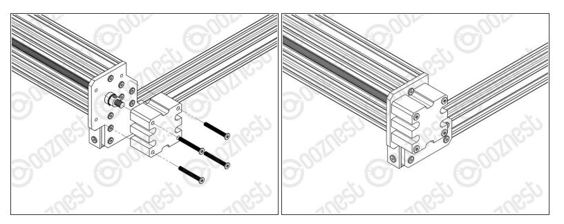
Onto the end of each ACME Screw attach an ACME-End-Cap using 4 x M5-Low-Profile-40mm bolts.
