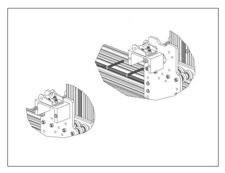
Secure the X-Axis-Moving-End-Assembly to the X-Plate-Back using 2 x M5-Low-Profile-60mm bolts and 2 x M5-Nyloc-Nuts.
