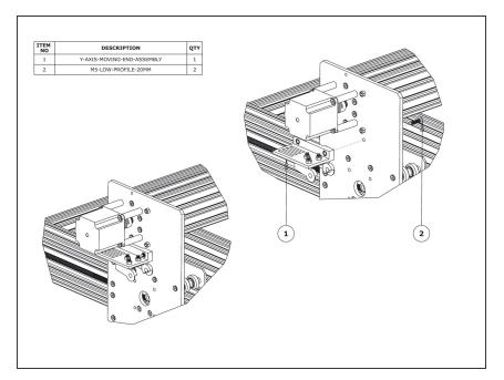
Secure the Y-Axis-Moving-End-Assembly using 2 x M5-Low-Profile-15mm bolts and the 2 x M5-Nyloc-Nuts already inserted into Y-Drag-Chain-Moving-End-Mount.
