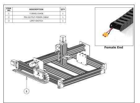
Lay the Y-Drag-Chain flat on a table. Feed the PSU-Output-Power-Cable through the whole length of the Y-Drag-Chain. Ensure that the end with the XT60-Connector, is located at the female end of the Y-Drag-Chain. (as shown in the 'Female End' image).
