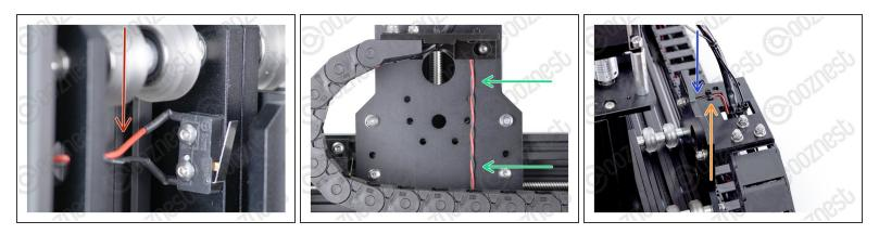
A Pull the Limit-Switch-2 Wire taught all the way from the switch to the Drag-Chain-Mount.
