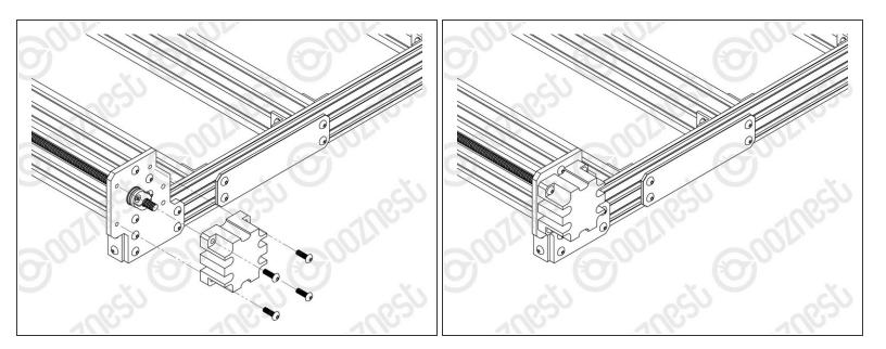
Using 12 x M5-Button-Head-Bolt-16mm attach 3 x Lead-Screw-Caps over the bare ends of the X & Y-Axis Lead-Screws.
