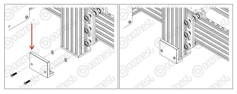
A Reference the correct face of the Height-Reference-Tool for your Router Head.
