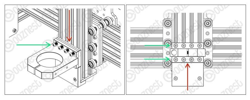
⚠ On one face of the Router-Clamp there are 4 threaded holes. These should be face down.
