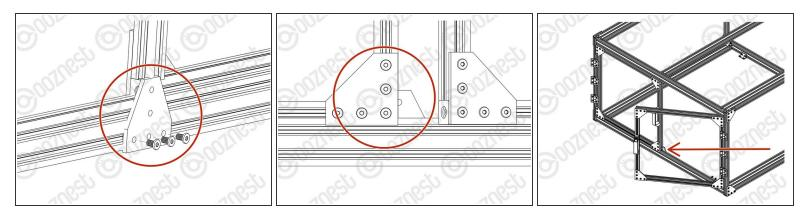
• Fix a T-Joining-Plate centrally to the bottom V-Slot-2040 Extrusion. This will function as a stop for the two doors.
