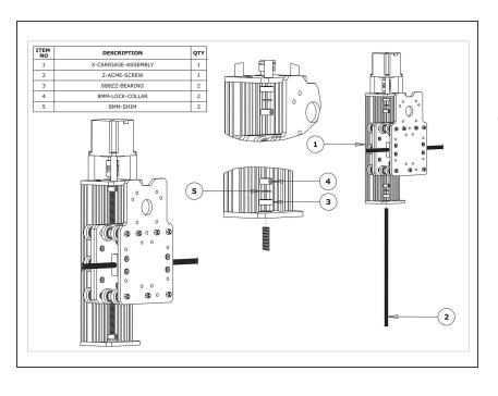
Slide the Z-ACME-Screw through the bottom of the Z-End-Mount-Bottom. Then slide on a 688ZZ-Bearing, 8mm-Shim, and a 8mm-Lock-Collar in this order.
