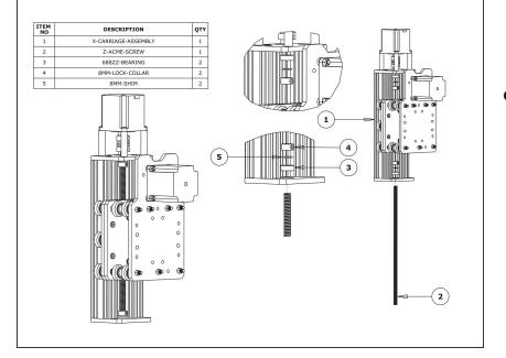
Slide the Z-ACME-Screw through the bottom of the Z-End-Mount-Bottom. Then slide on a 688ZZ-Bearing, 8mm-Shim, and a 8mm-Lock-Collar in this order.
