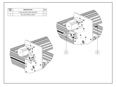
Secure the Y-Axis-Moving-End-Assembly using 2 x M5-Low-Profile-20mm bolts and the 2 x M5-Nyloc-Nuts already inserted into Y-Drag-Chain-Moving-End-Mount.
