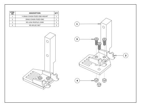
Attach a Drag-Chain-Fixed-End to the Y-Drag-Chain-Fixed-End-Mount in the orientation shown above, using 3 x M5-Low-Profile-15mm bolts and 3 x M5-Nyloc-Nuts.
