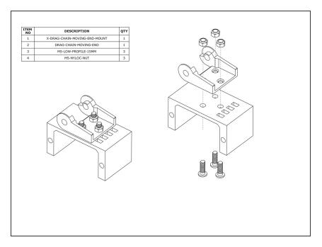
Attach a Drag-Chain-Moving-End to the X-Drag-Chain-Moving-End-Mount in the orientation shown above using 3 x M5-Low-Profile-15mm bolts and 3 x M5-Nyloc-Nuts.
