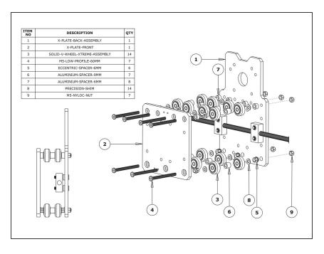
Run any piece of C-Beam extrusion in between the two rows of wheels. Initially, the C-Beam will wobble between the wheels. Turn the assembly upside down so the C-Beam WorkBee CNC Assembly 18 is sitting on the row of wheels with the Aluminium-Spacer-6mms.
