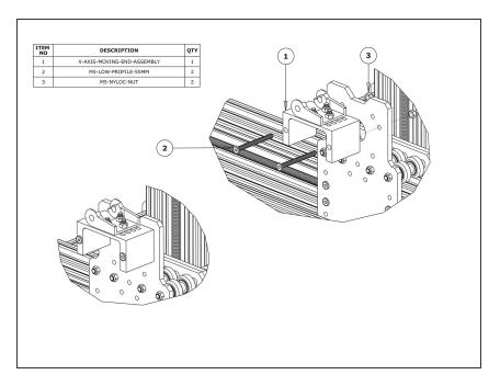
Secure the X-Axis-Moving-End-Assembly to the X-Plate-Back using 2 x M5-Low-Profile-55mm bolts and 2 x M5-Nyloc-Nuts.
